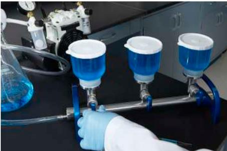
Additionally, since the device's end cap and hose barb can be setup in either orientation, all the valves are situated at the front of the manifold. This means there is no need to reach over the top of a filter funnel and maneuver behind a manifold to turn the valves on and off. Both features improve contamination prevention and reduce injury risk.
